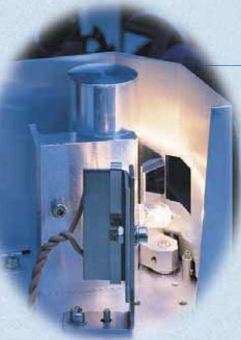
Lamps compartment thermally isolated from optical bench
